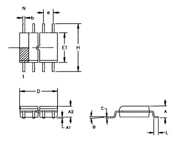
The chamfer on the body is optional. If it is not present, a terminal 1 identifier must be positioned so that  $\frac{1}{2}$  or more of its area is contained in the hatched zone.
